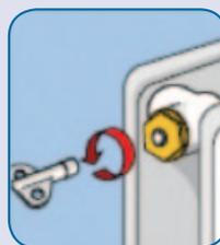
If you notice that a radiator is cool at the top, it may indicate that there is air in the system. This is a common issue, particularly in older houses or those which have suffered from low pressure. To release the air, first turn off the heating and allow the system to cool.
